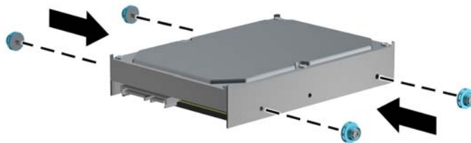
Figure 2-25 Installing Isolation Mounting Guide Screws in a 3.5-inch Hard Drive
